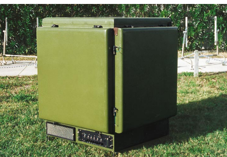
A full hemispherical coverage (C/S-band) array measuring 40 inches on a side provides three simultaneous receive beams or one transmit.
